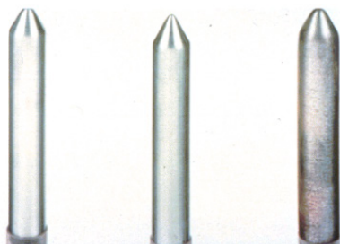
Figure 17: Schematic of the ISO 7120 steel corrosion test
