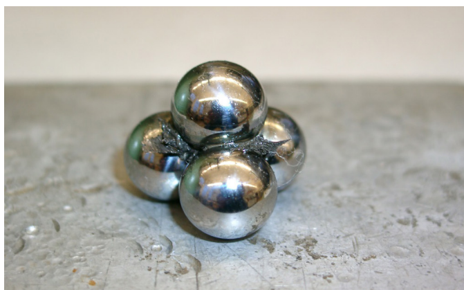
Figure 6: Four ball EP welding end of test specimen
